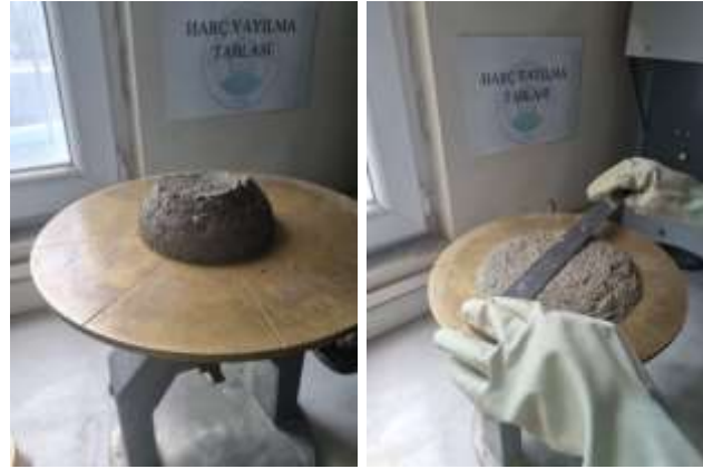
Figure 2. Flow table test
