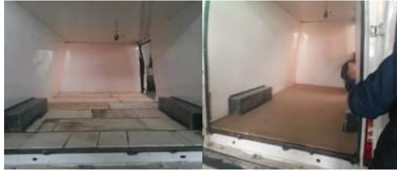
Figure 4. Application of Foam and Particleboard
