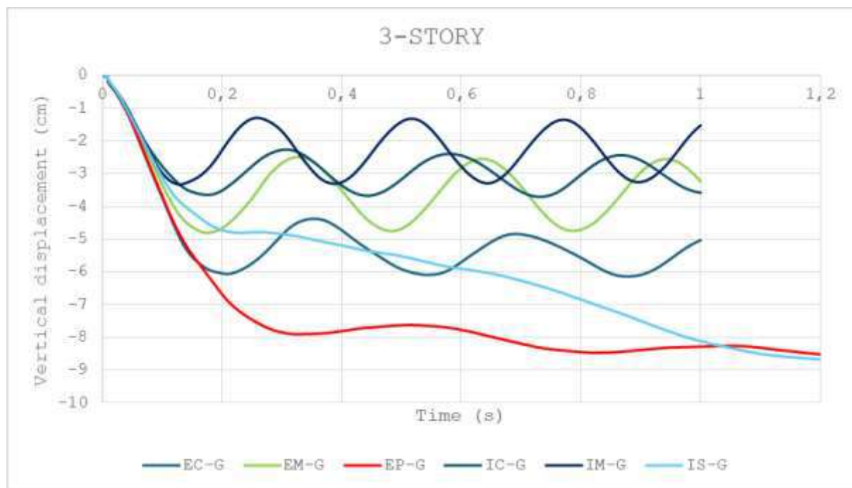
Fig. 6 Vertical displacements for both external and internal column removal scenarios on the ground floor of three stories.
