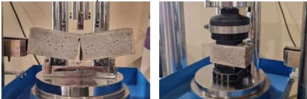
Figure 3. Flexural and compressive strength test
