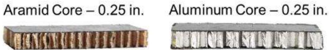
Fig. 1 Aluminum based sandwich structures with honeycomb cores [4]
