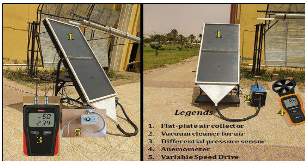
Figure. 1. Outdoor experimental setup of the solar air collector and measurement instruments.
