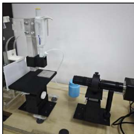
Fig. 2 Contact angle measurement device set-up for laser surface square-textured AA2024-T3 alloy
