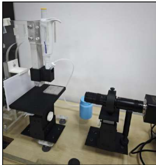
Fig. 2 Contact angle measurement device set-up for laser surface square-textured AA2024-T3 alloy
