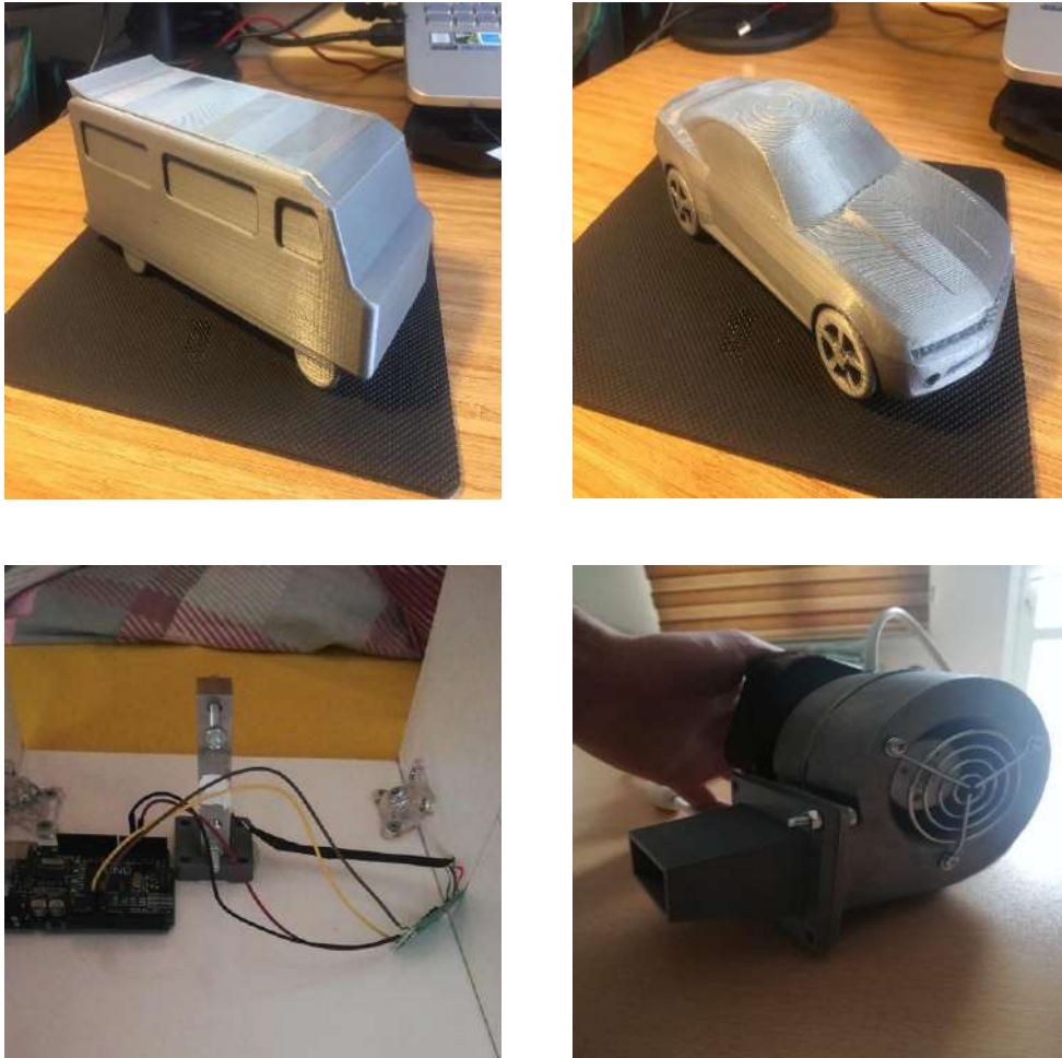
Fig. 2 Vehicle prototypes used in the experimental setup, mini wind tunnel (load cell setup) and snail fan
