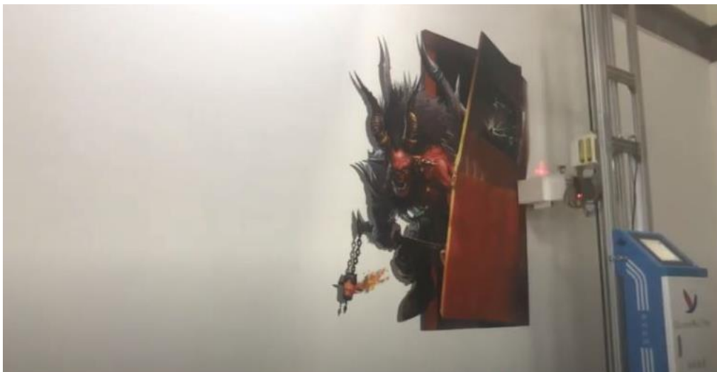
Figure 10 Painting machine capable of automatic three-dimensional printing on the wall
